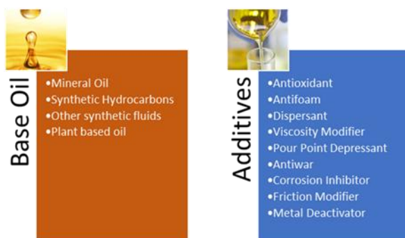
Figure 1. Lubricant - Base Oil and Additives
